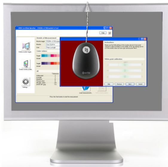
Fig. 5-5 Eye-One Display Placed on Screen
