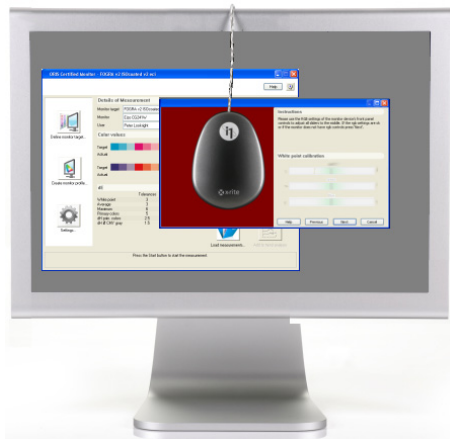
Fig. 3-4 Eye-One Display Placed on Screen
